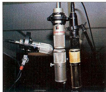
FIG. 1: The tube microphones were clustered tightly together so each could capture the same performance.
